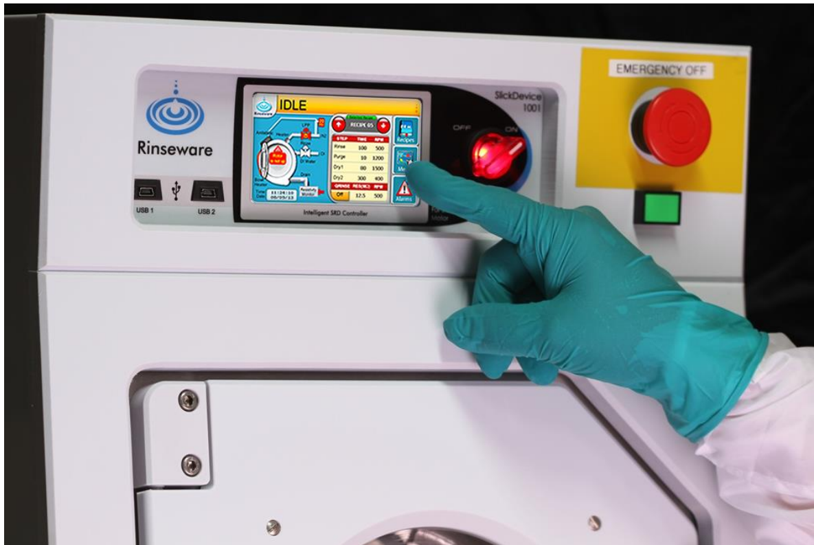
Figure 2. Rinseware SlickDevice 1001BL on a Semitool Single Stack 270 Spin Rinse Dryer
